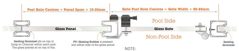
If using Gate Stiles, Gate Post hole Centres will be Gate width + 145mm.
